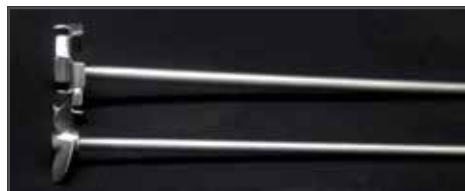
Propeller or dissolver for dispersing Carbopol polymers.
