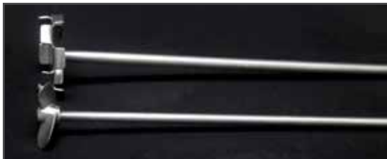
Propeller or dissolver for dispersing Carbopol® polymers.
