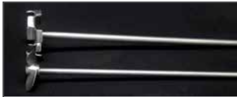
Propeller or dissolver for dispersing Carbopol polymers.
