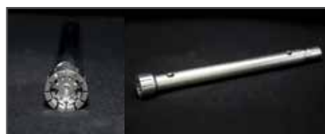
Homogenizer for preparing drug phase.
