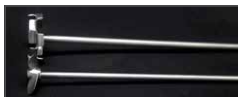
Propeller or dissolver for dispersing Carbopol polymers.
